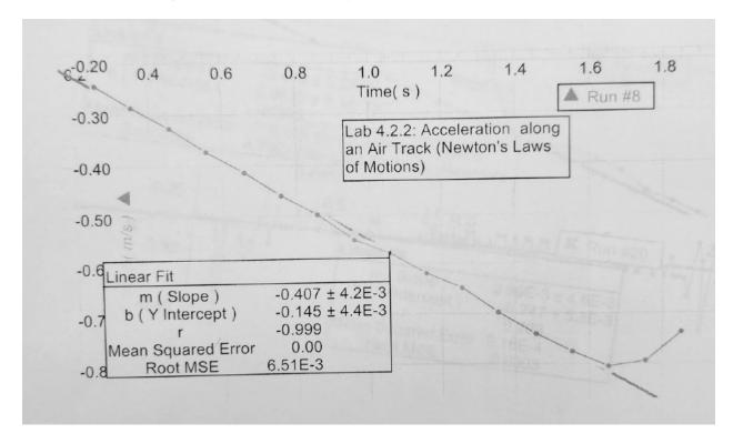
String Tension Along an Air Track: Velocity (m/s) vs. Time (s)
