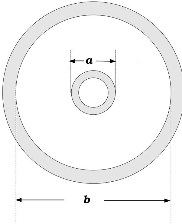
Figure 2: Cross section of the Cylindrical capacitor.
