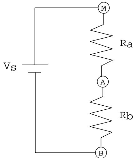
Figure 2: Voltage Divider.
