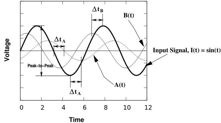
Figure 2: Sinusoidal signals  $I(t) = \sin(t)$ ,  $A(t) = 0.7 \sin(t + 1)$ , and  $B(t) = 0.4 \sin(t - 1)$ ; the phase differences, in the time domain, between  $I(t)$  and the other signals are labeled  $\Delta t_A$ , and  $\Delta t_B$ . The peak-to-peak range for  $I(t)$  is also shown. Note that phase differences may be easier and more accurate to measure between the signals' intersection with a common time axis rather than between their peaks.
