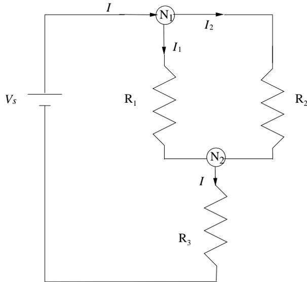
Figure 1: Test circuit: This figure shows the setup for Sections 8.3 and 8.4. Use the following values (or those provided by your instructor):  $R_1 = 10\text{k}\Omega$ ,  $R_2 = 5\text{k}\Omega$ , and  $R_3 = 1\text{k}\Omega$ .
