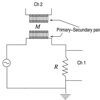
Figure 3: Diagram of the setup to examine the Mutual Inductance between coils; the number of turns of the secondary coil is  $N_s = 235$ ;  $R$  has a nominal value of 1 k $\Omega$ ;  $M$  is the Mutual Inductance.
