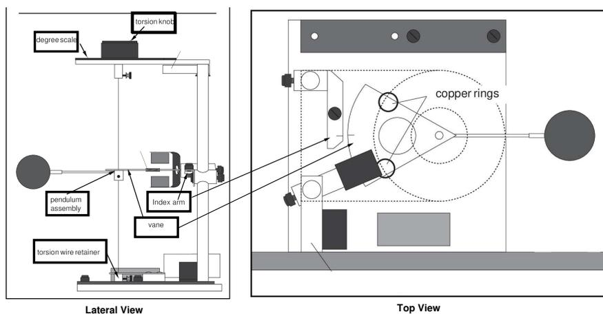
Figure 2: Torsion Balance; lateral and top views.
