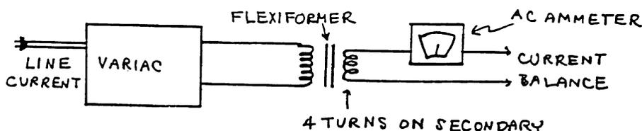
Figure 4: Circuit for supplying current to the balance.
