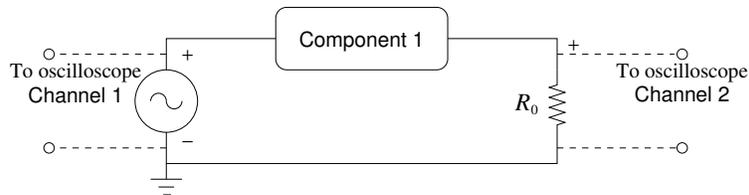
Figure 3: Base Circuit: Component 1 can be a Resistor,  $R$ , a Capacitor  $C$ , or an Inductor,  $L$ . Nominal values for these components are  $R = 1 \text{ k}\Omega$ ,  $C = 100 \text{ nF}$ ,  $L = 65 \text{ mH}$ , respectively. The nominal value for  $R_o$  is  $220 \Omega$ . The Signal generator is set to  $1 \text{ kHz}$  and  $2 \text{ V(p-p)}$ .
