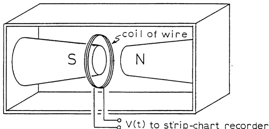
Figure 1: Diagram of setup for testing Faraday's Law.
