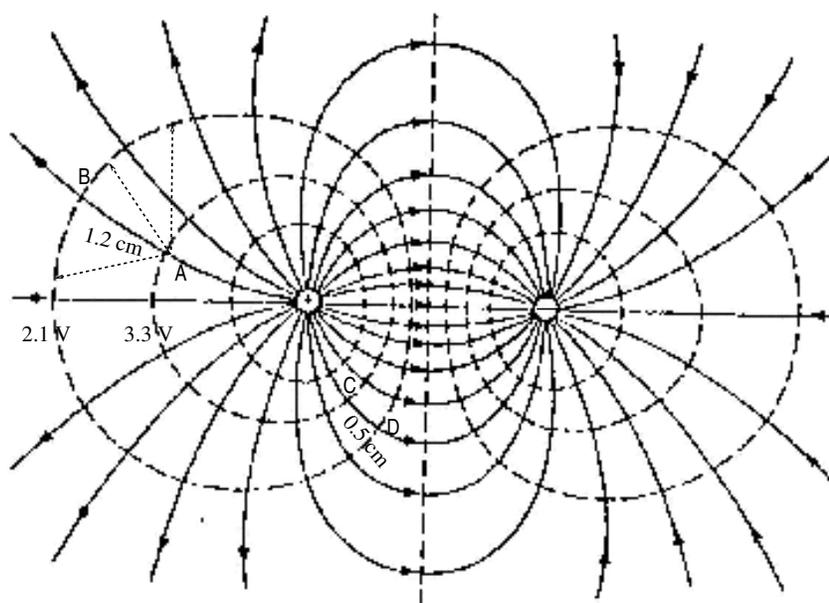
Figure 1: Contours of constant electric potential (equipotentials) and lines of the Electric Field between two point charges of equal magnitude and opposite polarity. The electric field lines are shown as solid lines pointing from high potential to low potential (indicated by arrows). The equipotentials are shown as dashed lines. The two sets of lines always intersect at right angles.
